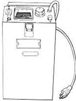
Figure 4-3 Typical portable dielectric test set.
